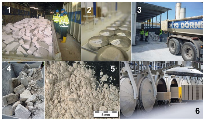
Fig. 2. Quality maintenance in the closed material cycle for AAC: sorted old AAC (1) is subjected to chemical and mineralogical spot checks by Xella T+F (2); old AAC, which fulfils our requirements, is delivered to an Ytong-factory (3), crushed (4) and fed back as granulate (5) into the production of AAC (6)
