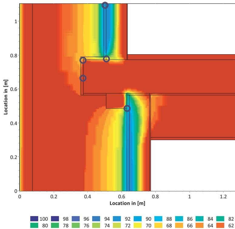
Fig. 8. RH distribution versus wooden floor-beam structure after 60 days under constant climatic conditions according to Table 2
