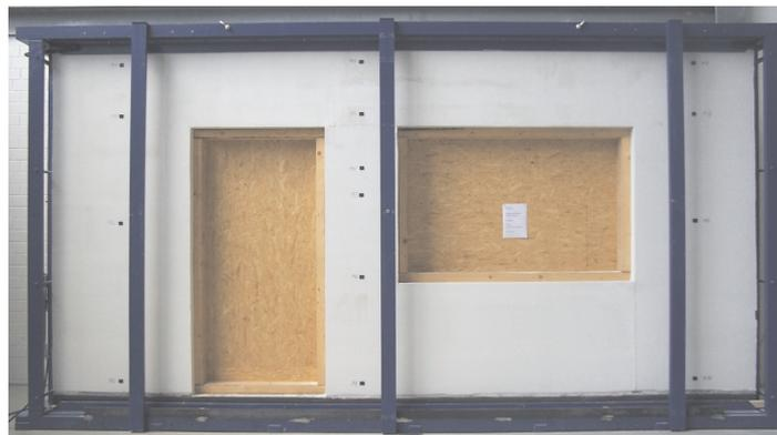
Fig. 3. Wall in bending test stand
